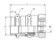
SKINTOP® GRIP-M is a double-strap strain relief cable gland with a high level of strain relief for harsh environmental conditions. Is is appropriate for portable equipment, cranes, conveying machinery, and systems on building sites.
