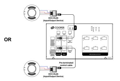
Connect the OCC-RJ45 Input/Output Device to the BMS system. Closure will be made across the Blue and Red wire locations. Connect a pre-terminated control cable between the REC/BMS/OUT RJ45 port on the Power Module and to one of the ports on the OCC-RJ45 ports.
