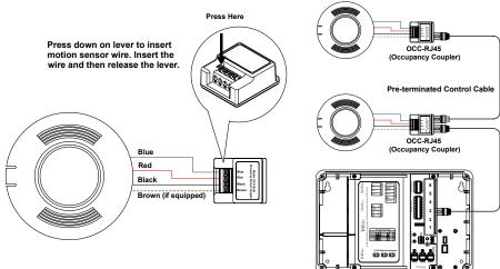
Connect the OCC-RJ45 Coupler to the BMS system. Closure will be made across the Blue and Red wire locations. Connect a pre-terminated control cable between the Receptacle/BMS Out RJ45 port on the Room Controller (port 5) or DLVP power module and to one of the ports on the OCC-RJ45 ports.
