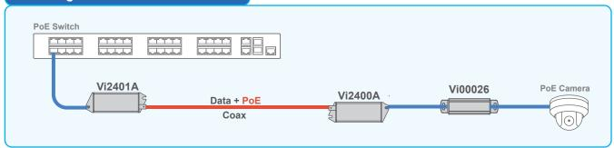
The Vi00026 requests maximum IEEE 803.2at PoE power from the PoE source to assure enough power for IP camera, extra power loss due to extended cable and Ethernet extenders regardless of camera rated power level.
