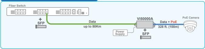
By using the SFPs, the Vi50000A will be compatible with most installed fiber types and can be directly connected to SFP modules installed in network switches.
