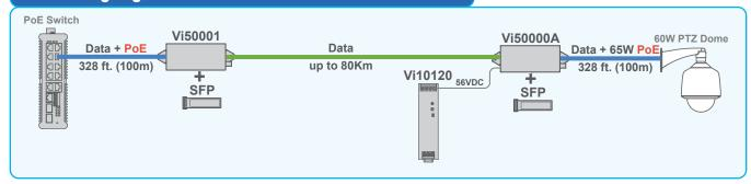
The Vi50000A is used with the Vi50001 for long distance high bandwidth applications. The Vi50000A provides up to 65W PoE power to meet the highest PTZ dome power requirements.
